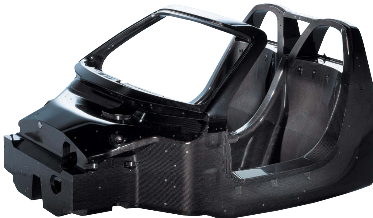
The Carrera GT's monocoque tub was the first Porsche to use such a construction method; it took five days to make a single tub
