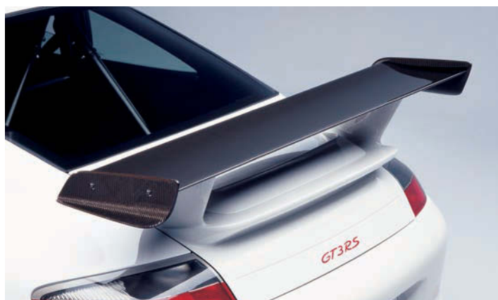
In 2004 the 996 GT3 RS was the first production Porsche to feature carbon-fibre parts, with the wing mirrors and fixed rear wing manufactured from the lightweight material
